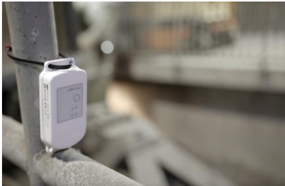
A temperature sensor, placed underground beneath the Chicago Loop (credit: Northwestern University)
